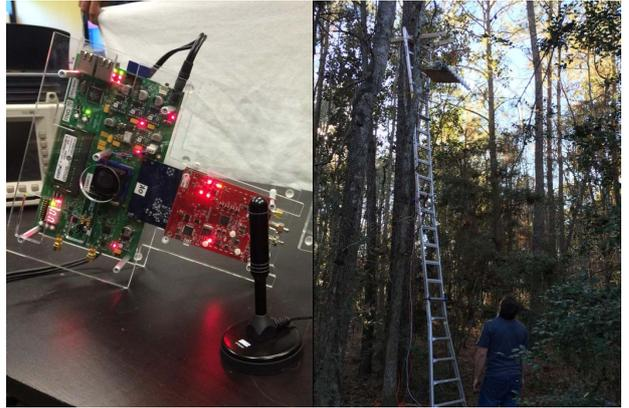
Fig. 4. Single-radio mobile node, omnidirectional antenna and outdoor installed AP.
